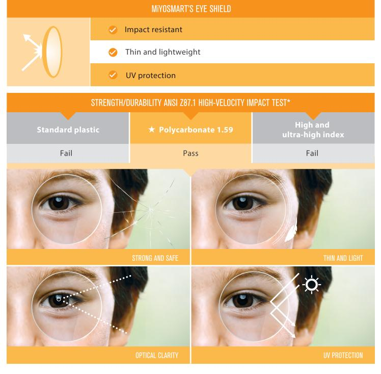
\*ANSI Z87.1 High Velocity Impact Test: The American National Standards Institure (ANSI) has established the most stringent impact and projectile penetration standards for ophthalmic lenses. The standard specifies that high impact lenses must pass "high velocity" testing where ¼" steel pallets are "shot" at the lens at a velocity of 150 feet-per-second. Polycarbonate passes ANSI Z87.1- the industry's highest standards for high-impact resistance ensuring full protection to every child.
